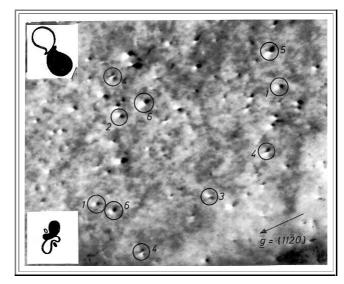
Same as before, but for a {1122} type specimen orientation. The observed contrasts match closely the calculated profiles for the types of dislocation loops assumed.
