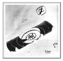
Several perfect stacking fault loops overlap (truncated by the sample surface, one of which has been preferentially etched; the etch pits at the dislocations are clearly visible). Some of the loops serves as nucleation sites for a second and third round of oxygen precipitation (shown as small coffee-bean like contrasts).
