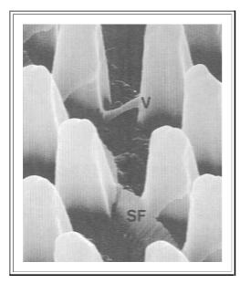
The structure marked "V" clearly results from a dislocation running from a trench to its neighbor.
