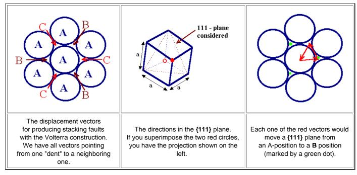
The relevant displacement vectors are of the type **b** = **a**/6<112>. (Check it! It's good exercise for getting used to lattice projections). Dislocations with this kind of Burgers vector are called **Shockley partial dislocations**, Shockley dislocations, or simply **Shockley partials**.
