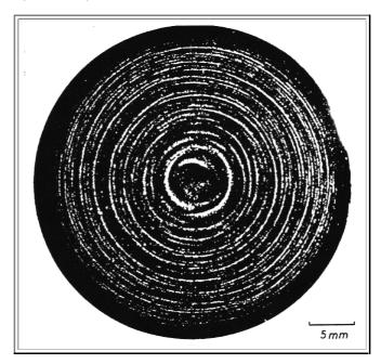
Looking at the etch pattern with a microscope at high magnifications shows that there are a lot of small defects (the B-swirls; white dots) and a much smaller number of larger defects (**A**-swirls; the black-white contrasts). Quantitative evaluation of the micrograph shows that the **B**-swirls are delineated as small and shallow pits whereas the **A**-swirls are delineated as hillocks.
