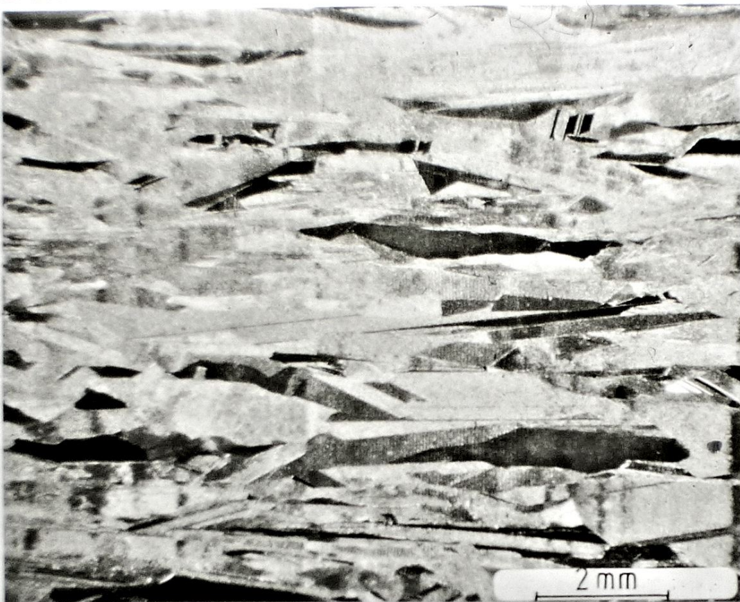
As - grown surface of a horizontally pulled S-Web ( KOH - etched )
