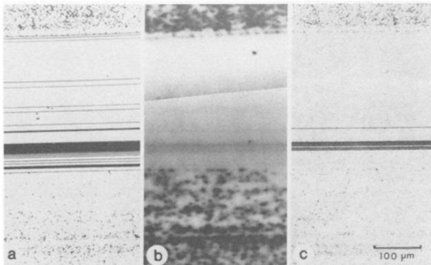
Fig. 10. Comparison between anodic etching at  $+0.5V$  (a), EBIC (b), and anodic etching at  $-0.4V$  (c) in ribbon-Si.
