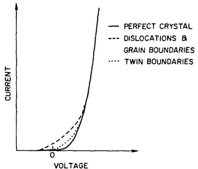
Fig. 11. Tentative current-voltage curves for various defects
