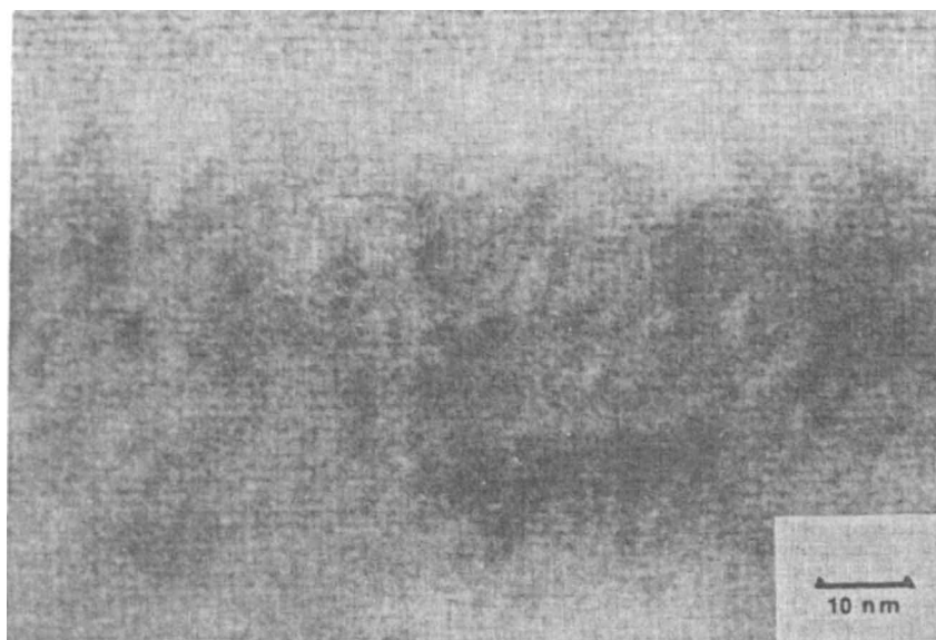
Image of a low-angle twist boundary on a \{100\} plane with a twist angle of 8^\circ taken under multi-beam conditions.
