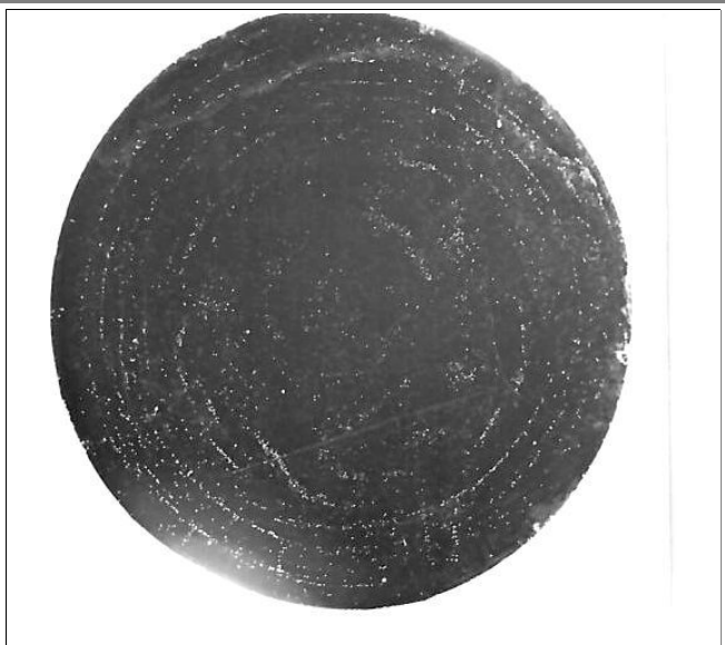
Etch pattern of swirl defects on a 33 mm float-zone (FZ) Si crystal; somewhat less showy than the one above..
