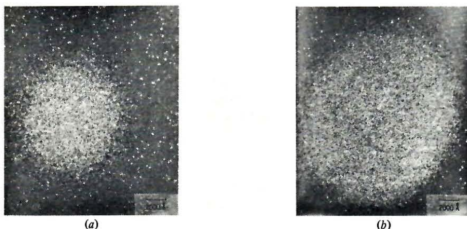
Figure 6. Weak-beam micrographs of the damage structure in 10 \Omega \text{ cm} p-type silicon at 20 K. The big white and dark spots are not due to irradiation but to sample preparation. (a) E_{\text{electrons}} = 600 \text{ keV} , dose \sim 5 \times 10^{22} \text{ electrons/cm}^2 , (b) E_{\text{electrons}} = 650 \text{ keV} , dose \sim 3.6 \times 10^{22} \text{ electrons/cm}^2 .
