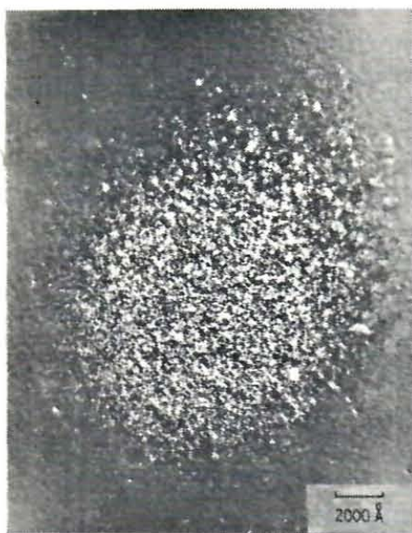
Figure 3. Weak-beam micrograph of 50 \Omega cm n-type silicon irradiated with about 5 \times 10^{22} electrons/cm 2 at 40 K.
