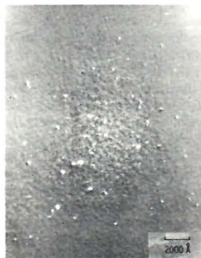
Figure 4. Weak-beam micrograph of 50 \Omega cm n-type silicon irradiated with about 5 \times 10^{22} electrons/cm 2 at 60 K. The big white spots are not due to irradiation but to sample preparation.
