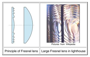
It wasn't so easy way back to shape glass like that. Nowadays it is easy, especially if you use plastic material and just press it into form. Fresnel lenses are no all over the place - as long as the ultimate in resolution doesn't matter. The "tips" at the singularities scatter light to some extent. and if you make the structure too dense, you run into diffraction effects at the periodic structure.
