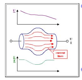
Current density **i** and field strength **E** may depend on the coordinates, because **U** and **I** depend on the coordinates, e.g. in the way schematically shown in the picture to the left. However, for a homogeneous material with constant cross section, we may write
