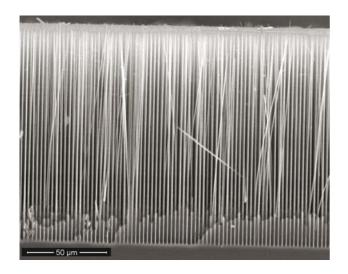
**Figure 2** SEM cross-section of nanowires (diameter about 0.9  $\mu$ m, lattice constant  $\approx 2 \mu$ m, length 140  $\mu$ m).
