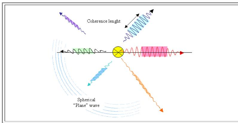
The picture might be interpreted as *photons* coming out of the light bulb. If one of those wavelets would be seen as a completely *abstract symbol* for a photon, this would be true. However, photons are *not* just short pieces of an electromagnetic wave, so one must not interpret this figure as a *picture* of photons.
