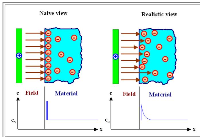
In a *naive* (and *wrong*) view, enough negatively charged carriers in the material would move to the surface to screen the field completely, i.e. prevent its penetration into the material. "Enough", to be more precise, means just the right number so that every field line originating from some charge in the positively charged plate ends on a negatively charged carrier inside the material.
