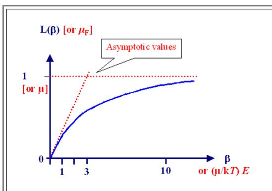
Since  $\beta$  is proportional to the field strength  $E$ , we see that the dipole moment and the polarization increases monotonically with  $E$ , eventually saturating and giving  $\langle \mu_F \rangle = \mu$  which is what we must expect.
