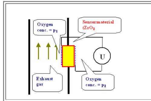
The sensor material experiences two different oxygen concentrations on its two surfaces, one of which is known (oxygen in air, a constant for all practical purposes), the other one is the concentration in the exhaust gas of a car which is supposed to be measured by the voltmeter
