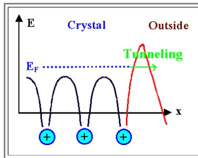
Now the **tunneling effect** may occur. It is a phenomenon inherent in quantum mechanics and allows electron "waves" to "*tunnel*" through a potential barrier.
