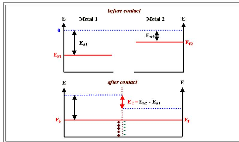
We have a dipole layer of charges at the interface which, owing to the large carrier density, is [extremely thin](#) and does not hinder current flow (it is easy for electrons to tunnel through the potential barrier).
