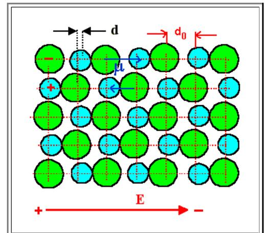
Orientation polarization results from minimizing the free enthalpy of an ensemble of (molecular) dipoles that can move and rotate freely, i.e. polar liquids.
