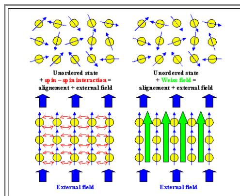
Of course, if the material you are looking at *is* a real ferromagnet, you don't have to *pretend* that there is a built-in magnetic field, because there *is* a large magnetic field, indeed. But this looks like mixing up cause and effect! What you want to result from a calculation is what you start the calculation with!
