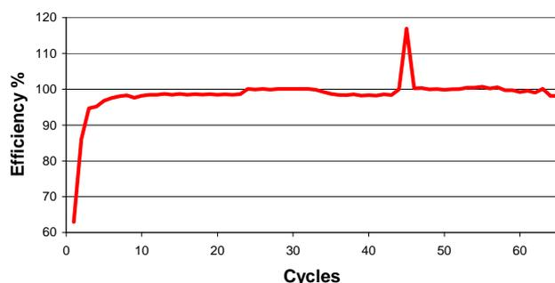
**Figure 3** Anode charge/discharge efficiency in a half-cell. Shown is the difference between discharge and charge vs. cycle number. The peak around cycle 45 is an artifact caused by a failure of the temperature control.
