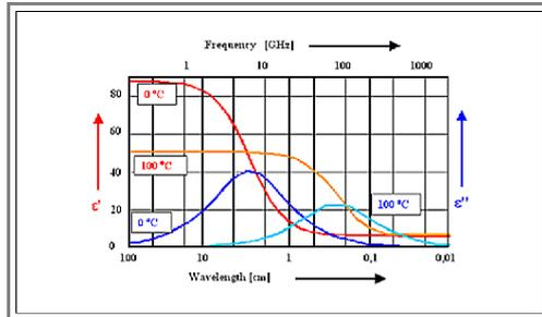
The polarization mechanism is orientation polarization, we expect large imaginary parts of the dielectric function in the **GHz** region.
