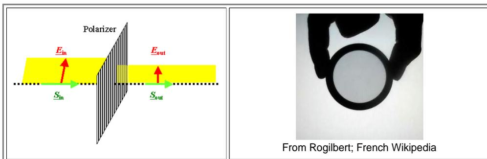
Turn your polarizer and the light intensity coming out stays either constant if the incoming beam is not polarized at all (but is always lower in intensity) or varies between zero and maximum (=incoming) intensity in a  $\cos^2$  fashion if the incoming beam is **100 %** linearly polarized, as shown above. If the beam is *partially* polarized you have a mix of the two extremes.
