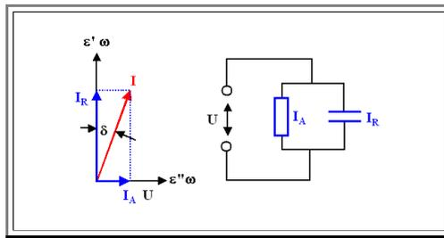
The pointer diagram for an *ideal* dielectric  $\sigma(\omega = 0) = 0$  can always be obtained from an (ideal) resistor  $R(\omega)$  in parallel to an (ideal) capacitor  $C(\omega)$ .
