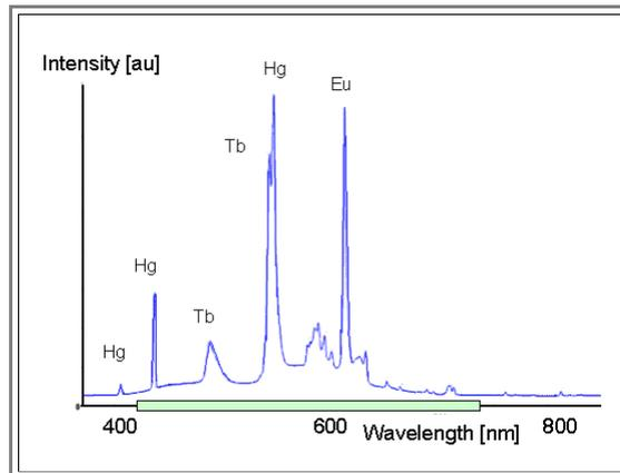
● The picture makes clear why luminescence can have a high efficiency: A lot of the energy going in comes out as light with sharp frequencies in the visible range. There is no need to always produce a lot of infrared and ultraviolet light in the process.
