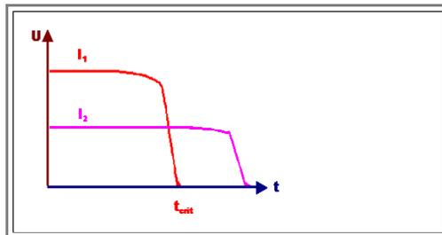
The voltage needed to press your tiny test current through the dielectric starts to decrease rapidly after some time - hours, days, weeks, ..., and this is a clear indication that your dielectric becomes increasingly leaky, and will go up in smoke soon.
