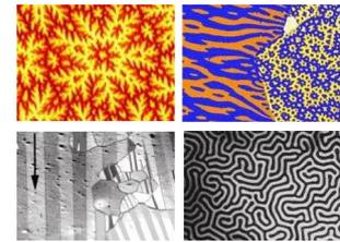
For ferromagnetic materials in an external magnetic field, energy can be gained by increasing the total volume of domains with magnetization as parallel as possible to the external field - at the expense of unfavorably oriented domains.
