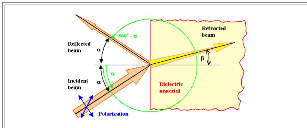
In essence we have an incoming beam, a **reflected beam** and a **diffracted beam** that "goes" into the material.
