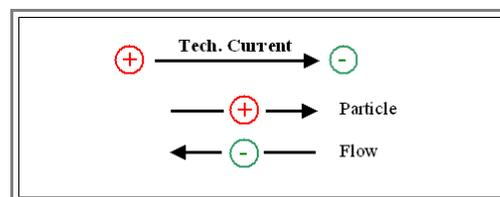
In words: A technical current  $I$  flowing from + to - may be obtained by *negatively* charged carriers flowing in the *opposite* direction (from - to +), by *positively* charged carriers flowing in the *same* direction, or from both kinds of carriers flowing at the same time in the proper directions.
