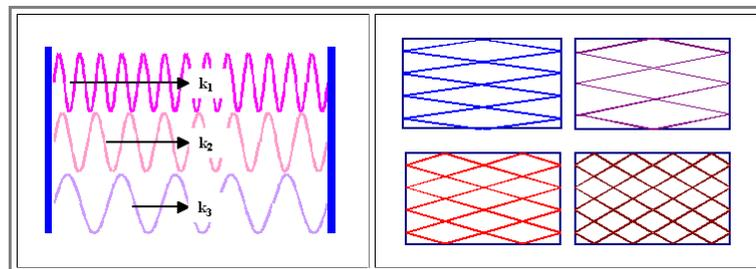
A musical instrument that isn't long and slender like an organ pipe or a flute (i.e. an essentially 1-dim. system) but a rectangular box (or a complex-shaped body shape like a violin, can contain standing waves in all directions with many possible wavelengths. Same for our Laser; cf.. the situation in the figure on the upper right.
