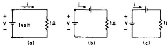
Fig. 3. “Impedance” seen by the labeled battery is  $1 \Omega$  in (a), apparently  $\frac{1}{2} \Omega$  in (b), and apparently infinite in (c).
