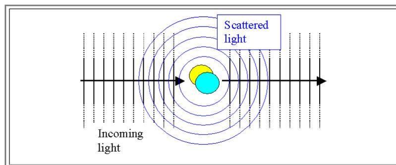
If we relate the total power (= energy per second) **P<sub>sc</sub>** contained in the scattered part to the intensity **I** = power per **cm<sup>2</sup>** contained in the incoming beam, i.e. from **P<sub>sc</sub>/I = σ**, the quantity **σ** has the dimension **cm<sup>2</sup>** and is therefore called the **scattering cross section**.
