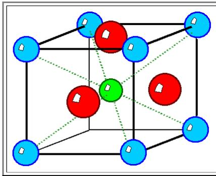
Often, the lattice is not exactly cubic, but slightly distorted. In the case of **BaTiO<sub>3</sub>** this is indeed the case: The **Ti** - ion does not sit in the *exact* center of the slightly distorted cube, but slightly off to one side. It thus has *two* symmetrical positions as schematically (and much exaggeratedly) shown below
