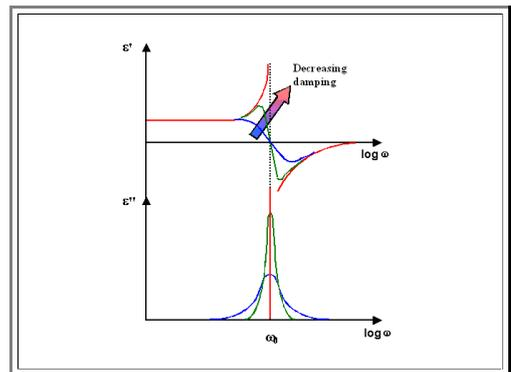
The complete frequency dependence of the dielectric behavior of a material, i.e. its dielectric function, contains all mechanisms "operating" in that material.
