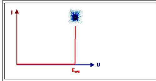
After reaching  $E_{crit}$ , a sudden flow of current may, within very short times ( $10^{-8}$  s) completely destroys the dielectric to a smoking hot mass of undefinable structure.
