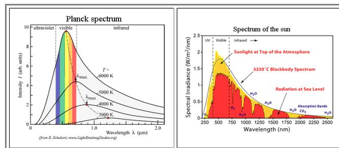
The sun comes pretty close to a black-body spectrum and the same is true for a light bulb or any other light source relying on high temperatures.
