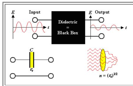
As long as our system is linear ("twice the input  $\Rightarrow$  twice the output), a sinewave going in will produce a sinewave coming out, i.e. the frequency does not change.
