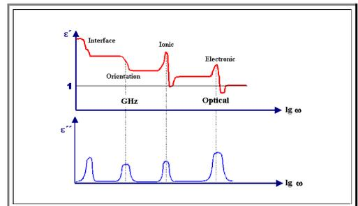
A widely used diagram with all mechanisms shows this, but keep in mind that there is no real material with all 4 major mechanisms strongly present!
