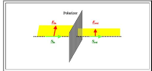
General case: *elliptical* polarization; important are the two extremes: *linear* and **circular** polarization.
