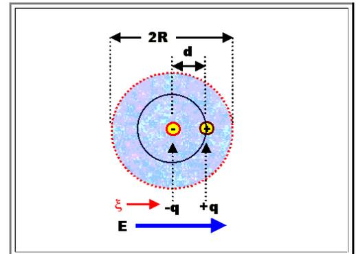
Ionic polarization describes the net effect of changing the distance between neighboring ions in an ionic crystal like **NaCl** (or in crystals with some ionic component like **SiO<sub>2</sub>**) by the electric field
