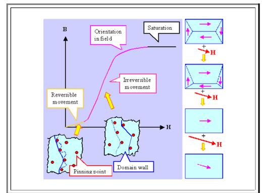
Depending on the shape of the hysteresis curve (and described by the values of the remanence  $M_R$  and the coercivity  $H_C$ ), we distinguish hard and soft magnets  $\Rightarrow$ .
