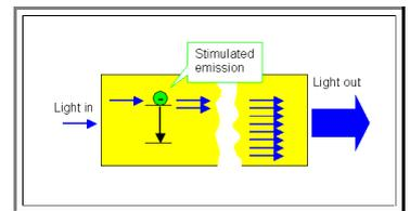
Second we need **s**timulated **e**mission, a phenomenon that was calculated and predicted by **Albert Einstein** in **1916**. In simple terms, stimulated emission means that a photon with the energy  $\Delta E$ , when encountering an electron sitting on the upper energy level, stimulates it to "fall down" and to emit a photon that is identical in wave vector, and phase to the one that stimulates the process (and does not get absorbed!)
