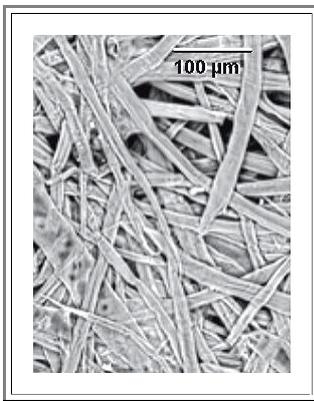
The paper, for example, is not perfectly flat but has a roughness on some length scale far larger than the wavelength of light, but smaller than what your eye can easily resolve as shown in the picture. Some parts of it thus are always reflecting the light into your eye.
