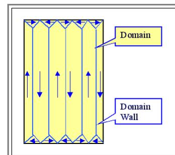
Both domain structures *decrease* the external field and thus  $W_{\text{field}}$  because the flux lines now can close inside the material. And we kept the alignment of the magnetic moments in most of the material, it only is disturbed in the domain walls. Now which one of the two configurations shown above is the better one?
