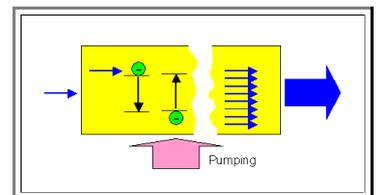
**Pumping** requires that we put plenty of energy into the system all the time. This can be done by intense illumination (obviously with light of somewhat higher energy than  $\Delta E$ ). Some Lasers of the US military were supposed to be pumped by **X-rays** produced by a nuclear explosion (no joke). They would not live long but still be able to produce a short-lived ultra-high intensity Laser beam suitable for shooting down missiles.
