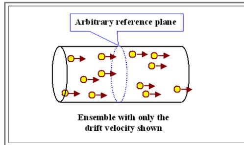
We now equate the *current density* with the *particle flux density* by the basic law of current flow:
