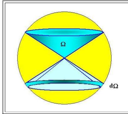
Relations with spherical symmetry where the value of  $\Theta$  does not matter - i.e. it does not appear in the relevant equations - are more elegantly expressed with the solid angle  $\Omega$ .
