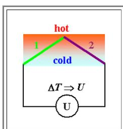
Lets look at a typical situation: We have a thermocouple mader with a material 1 and a material 2. It's "contacted" by whatever (material 3, black lines). The junction of material1 and material 2 is hot, the rest is cold (and has the same temperature).
