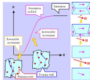
Depending on the shape of the hystereses curve (and described by the values of the remanence  $M_R$  and the coercivity  $H_C$ ), we distinguish hard and soft magnets  $\Rightarrow$ .
