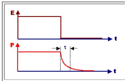
In formulas, we expect that  $P$  decays starting at the time of the switch-off according to
