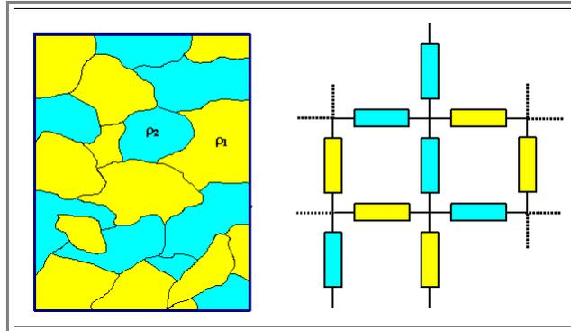
But no matter what kind of volume fraction you use and how you treat the resistor network - the resulting resistivity will **never** be smaller than that of the ingredient with the smallest resistivity.
