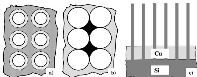
**Figure 1** a) Schematic top view of macropores (diameter around 2  $\mu\text{m}$ ) and their enlargement by chemical etching (dashed lines), b) Formation of nanowires (black) by overlap of the enlarged pores. c) Schematic cross-section with the Cu layer (thickness  $> 10 \mu\text{m}$ ).
