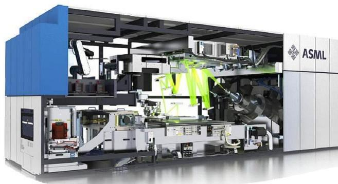
That is the kind of "projector" that will move into chip production after lenses have reached the *end of the art*. It needs to operate in vacuum because air starts to absorb light below around **185 nm**.
