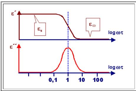
Note that  $\omega$  for curves like this one is always on a *logarithmic scale!*
