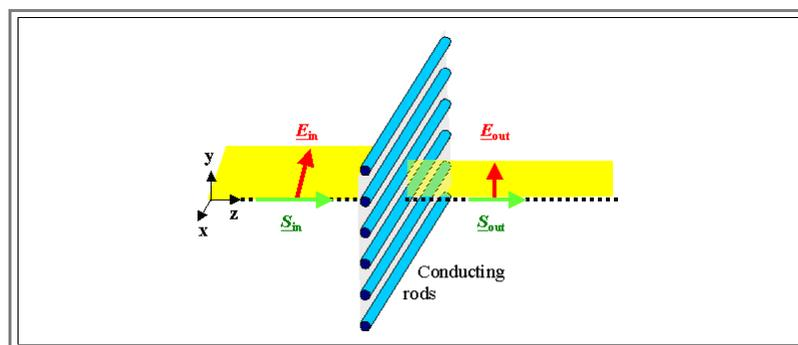
**Surprise!** The polarization direction is *not* parallel to the rods as one would naively imagine but **perpendicular** to it.
