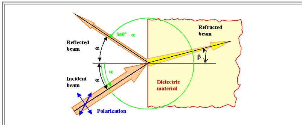
In essence we have an incoming beam, a **reflected beam** and a **diffracted beam** that "goes" into the material.
