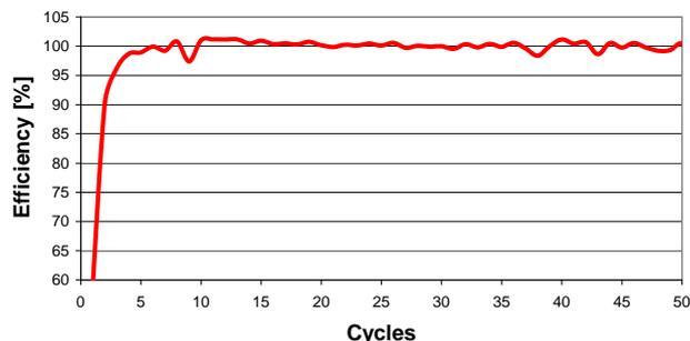
**Figure 5** Charge/discharge efficiency vs. cycle of first battery.
